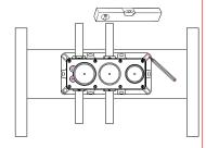
Put the installation box on the wood plate. Measure the correct position with level and marks.
