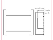
Fix a wood plate to the two wood pipes for faucet installation.
