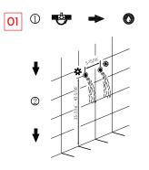
Flush the water supply lines throughly to drain debris and impurities. Shut off the water before installation.
