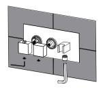
Install the handles and connector with allen keys. Test and make sure all the functions are closed when handle is pointed at OFF position.
