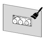
Create a dry wall around the installation box and brush with water proof glue.
